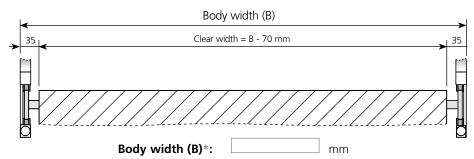
\* Indications from 2250 - 3000 mm in 50 mm steps possible. (Clear width: 2280 - 2630 mm)
